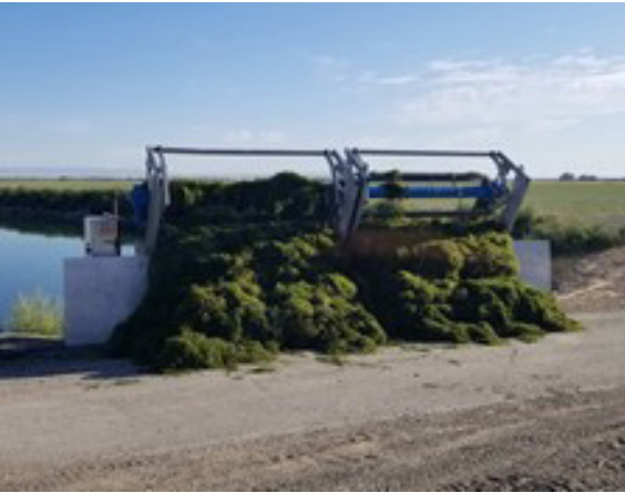
FlexRake handles the heavy inflow of moss from the lake
