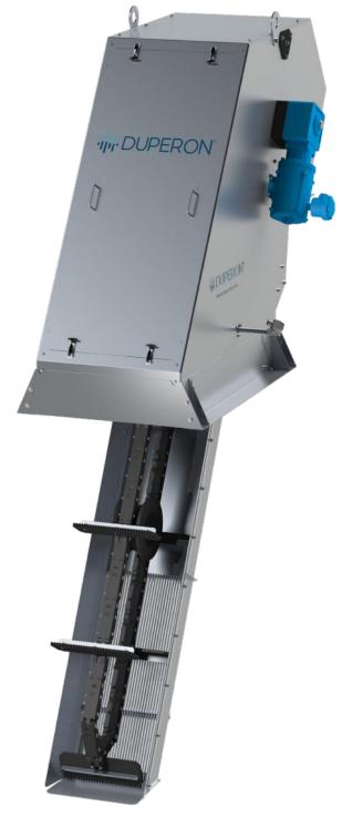
The FlexRake<sup>®</sup> Low Flow is a front-clean, frontreturn mechanical bar screen. It features the SmartLink <sup>™</sup> multifunctional link system, which eliminates underwater sprockets, bearings or tracks. The groundbreaking flex/pivot action of the Duperon<sup>®</sup> FlexRake<sup>®</sup> is unhampered by large debris. It is offered in a range of channel widths, depths and bar openings to meet the needs of small communities.
