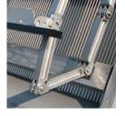
The FlexLink<sup>™</sup> forms its own rotating framework at the bottom of the channel.
