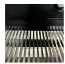
Scrapers remove debris from the face of the wedgewire screen.
