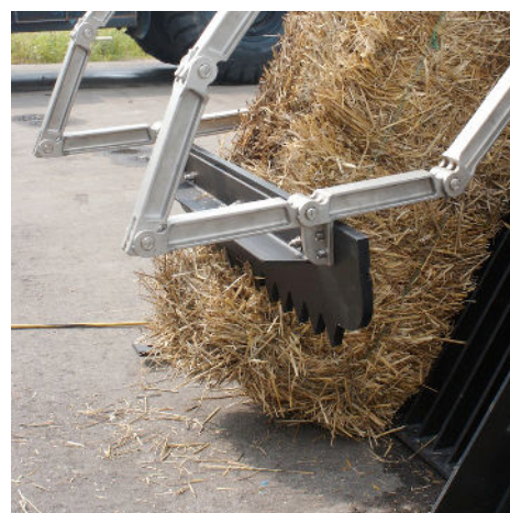
Figure 1. The investment cast links on the FlexRake HD and Harvest Rake function as a frame, lower sprocket, and connection point for scrapers. Since they are not limited to a fixed path of travel, in addition to eliminating the risk of jams, the links also allow the raking mechanism to pivot and capture large or irregular shaped debris.
