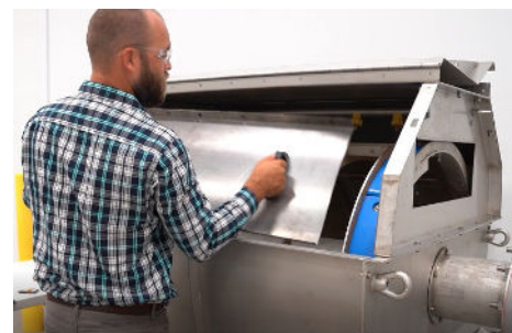
Figure 1. The removable panels on the Duperon drum screen allow operators to easily access the internal chamber for faster cleaning. It is designed to stand at chest height, so operators can perform scheduled or as-needed cleaning with minimal risk of injury and no need for a confined space entry. In addition, once cleaning is complete, the panel can be quickly reinstalled with common tools and will fully seal to eliminate any chance of leaking.
